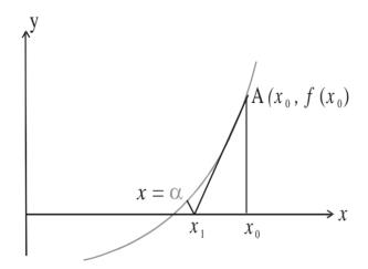
In this method, instead of taking two initial rough approximations to the root  $x = \alpha$  as in the previous two methods, a single rough approximation  $x_0$  to the root is taken. Then we use the following formula, known as Newton-Raphson formula or Newton iteration formula, to get the successive approximations.
