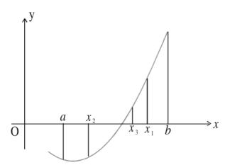
if f(x) = 0, then  $x_1$  is the root of equation f(x) = 0. Otherwise the root lies between a and  $x_1$  or  $x_1$  and b according to  $f(x_1)$  is positive or negative. Then we bisect the interval and continue the process until the root is found to desired accuracy.
